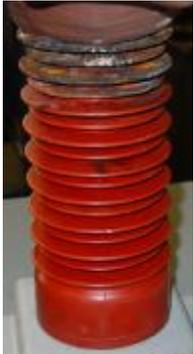
*Tracking on switchgear insulator.*
